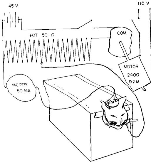
FIG. 1. Diagram of the wiring employed, permitting an interrupted current of determined amperage to be applied through an animal's head to determine the threshold for convulsions. (Reproduced with permission from ref. 2.)
